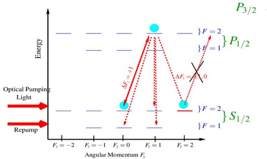
**FIG. 1.** Outline of the optical pumping process including the steps in the biased random walk. The quantum number  $F$  is the combined nuclear and atomic angular momentum. The stretched state is highlighted in red.
